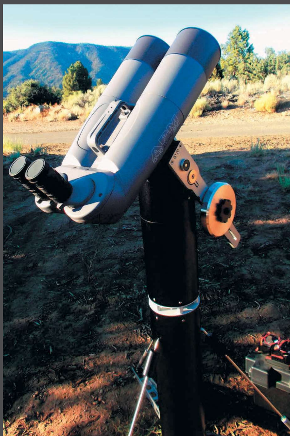
Image 3 - The TTS-160 is capable of payloads to 50 pounds, yet weighs just 30 itself.
